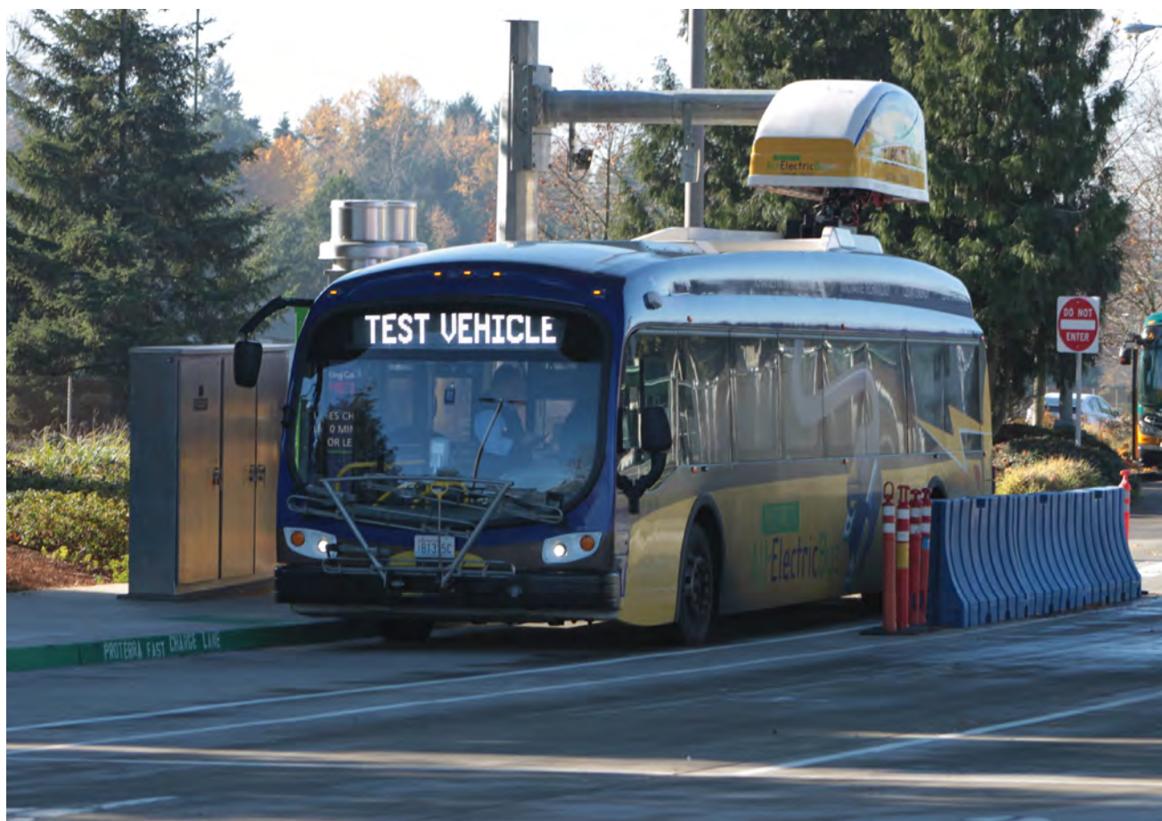
A contactless electric bus charging station in Washington state. Credit: Creative Commons/SounderBruce, CC BY-SA 2.0
